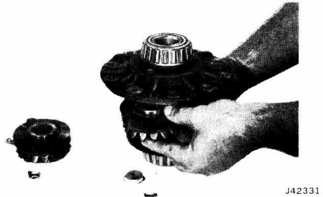
Fig. 10-71 Removing Side Gear and Clutch Pack
