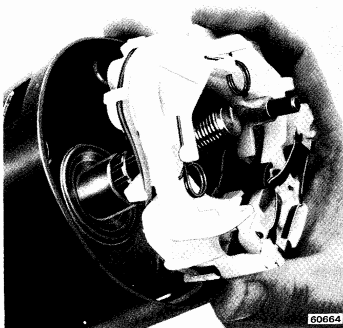
Fig. 11-8 Removing-Installing Turn Signal Switch
