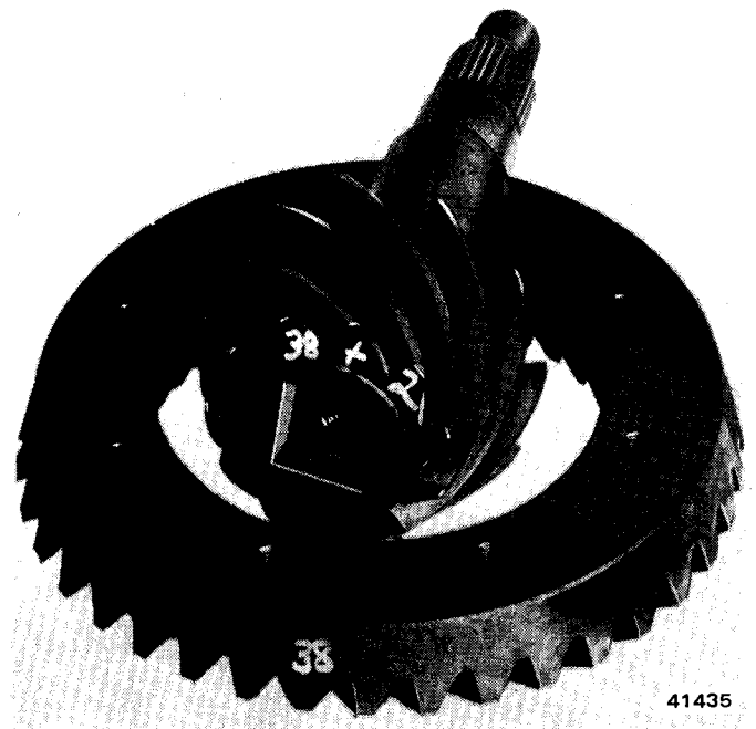
Fig. 10-41 Ring and Pinion Gear Markings
