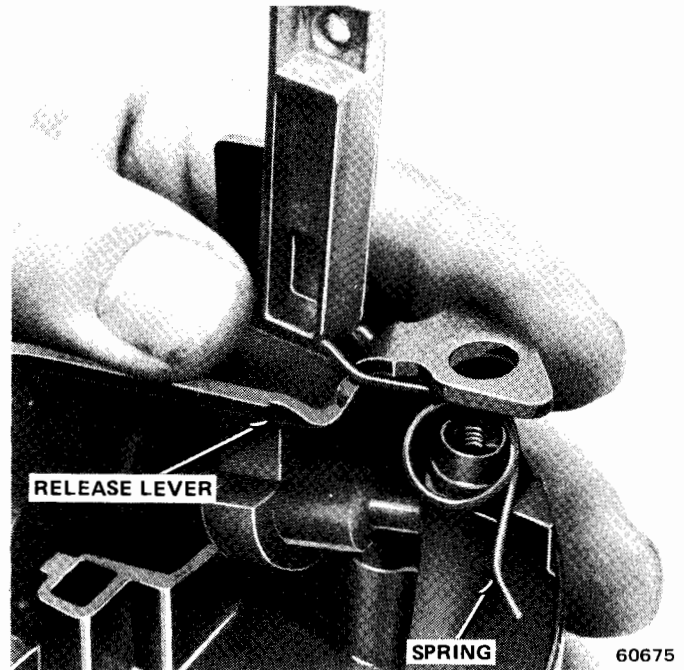
Fig. 11-21 Installing Release Lever and Spring
