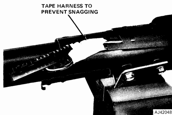
Fig. 11-29 Signal Switch Harness Removal
