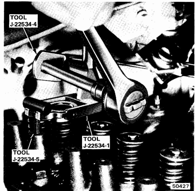
Fig. 1A-10 Valve Spring Removal
