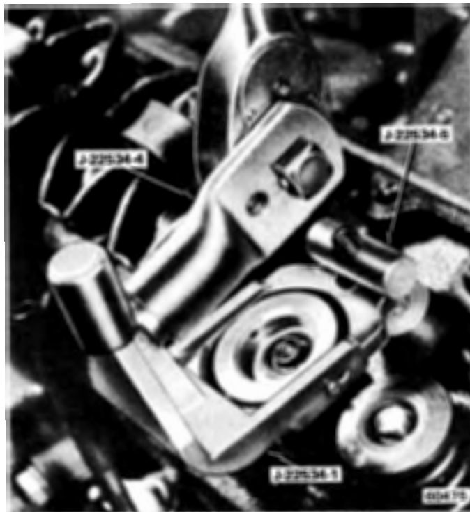
Fig. 1B-10 Valve Spring Removal
