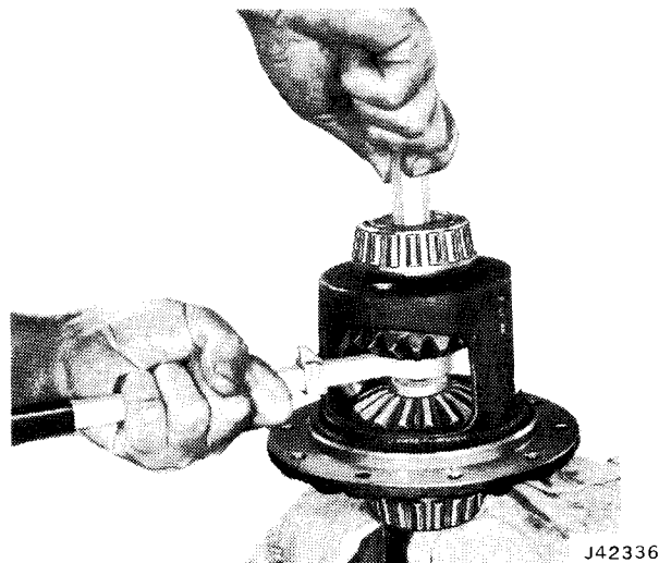
Fig. 10-75 Threading Forcing Screw into Rotating Tool
