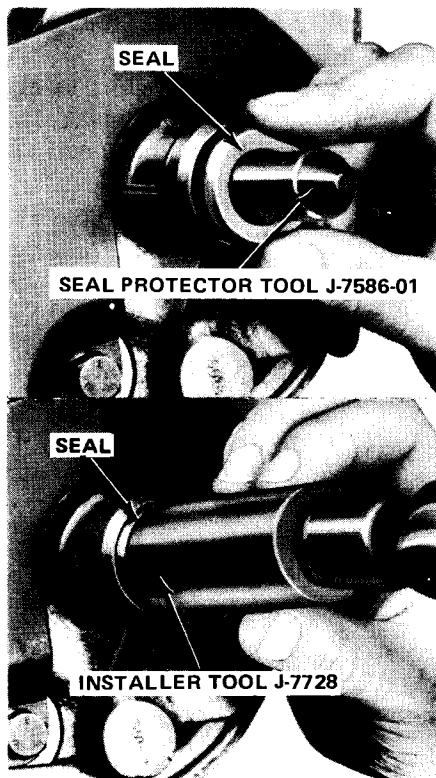
Fig. 11-98 Installing Pump Shaft Seal
