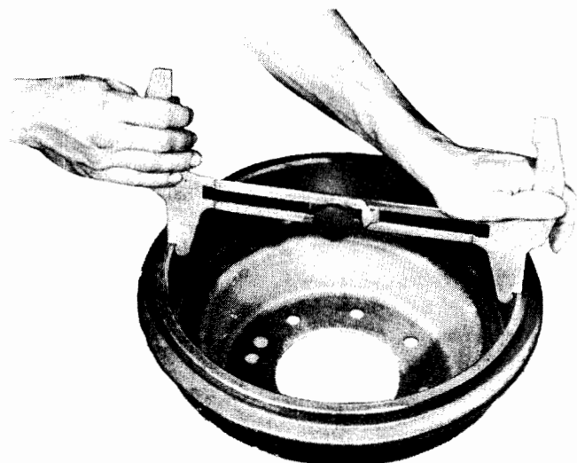
Fig. 9-19 Using Drum-to-Lining Clearance Gauge
