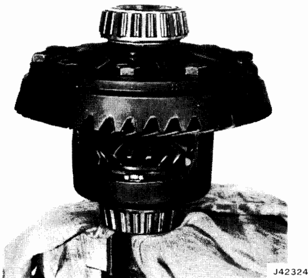
Fig. 10-65 Differential Mounted on Axle Shaft
