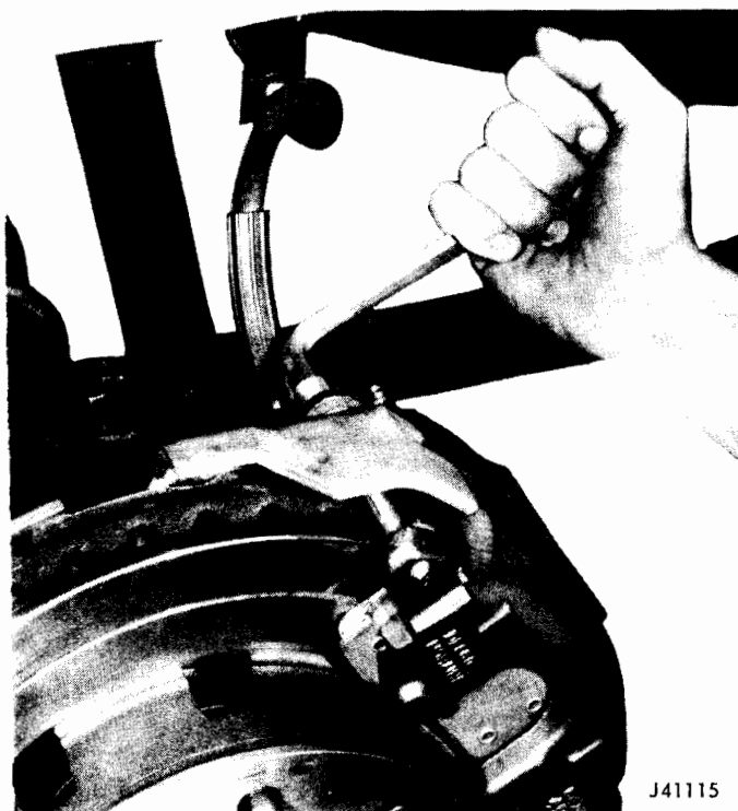
Fig. 9-29 Removal of Caliper Mounting Bolts
