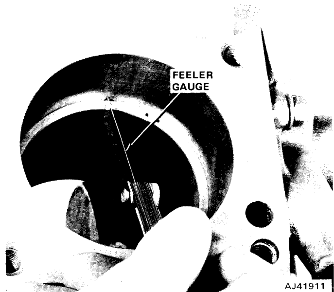
Fig. 1A-41 Ring Gap Clearance
