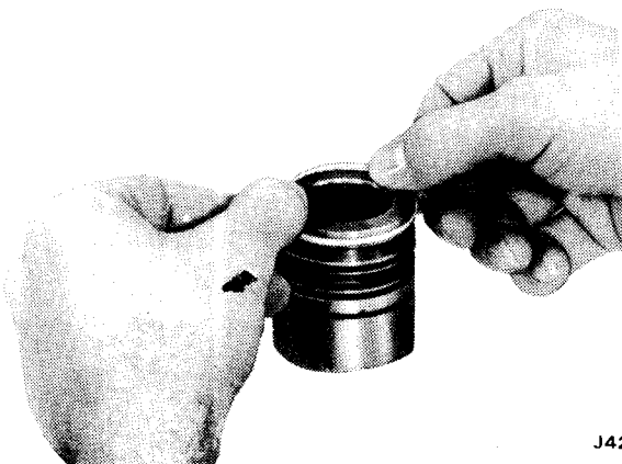
Fig. 11-87 Installing Valve Seal Rings
