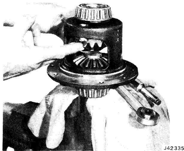
Fig. 10-74 Installing Clutch Pack and Side Gear
