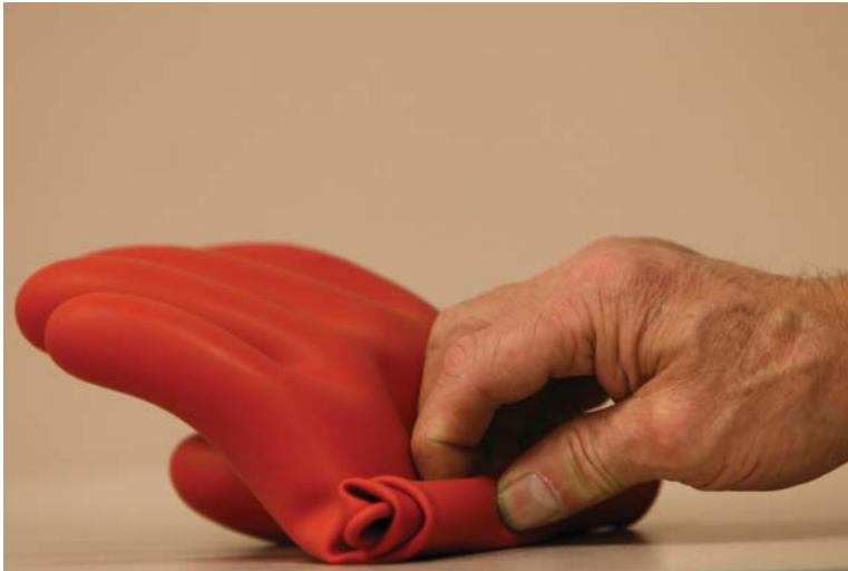
FIGURE 1-30 Test the isolation gloves for leaks before each use.
