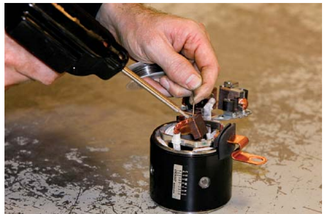
FIGURE 6-30 Soldering a new brush to the field coil lead.
