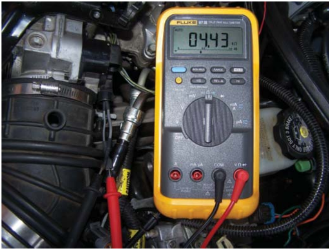
FIGURE 3-29 Using an ohmmeter to test the continuity between terminals A and C of a potentiometer.
