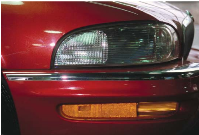
FIGURE 8-38 Cornering lights are used to provide additional illumination during turns.
