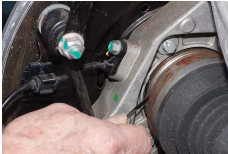
FIGURE 10-29 Measuring the air gap.
