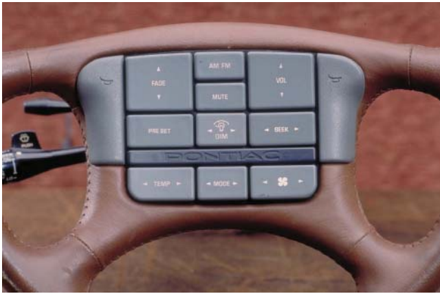
FIGURE 14-97 Audio system with steering wheel-mounted remote control.
