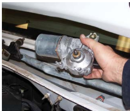
P24-8 Remove the motor.
