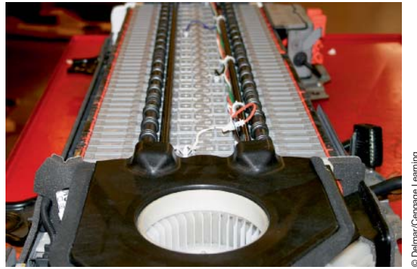
FIGURE 5-21 Battery pack made of several prismatic cells.
