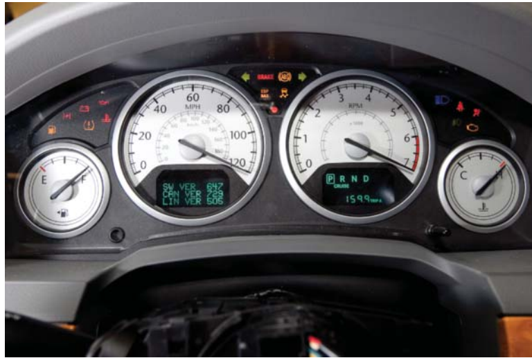
FIGURE 13-2 All EIC segments are illuminated during the prove-out display.
