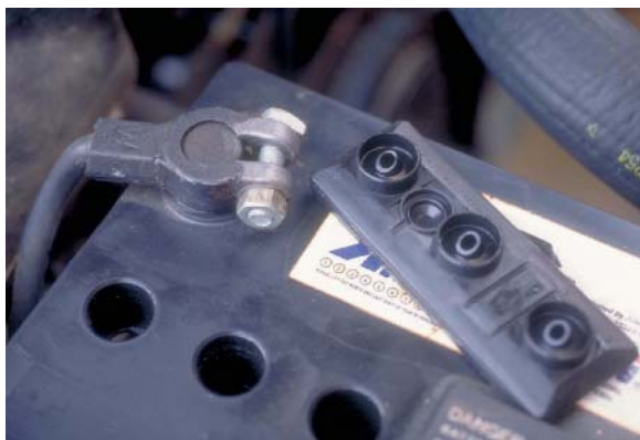
FIGURE 5-7 The vents of a conventional battery allow the release of gases.
