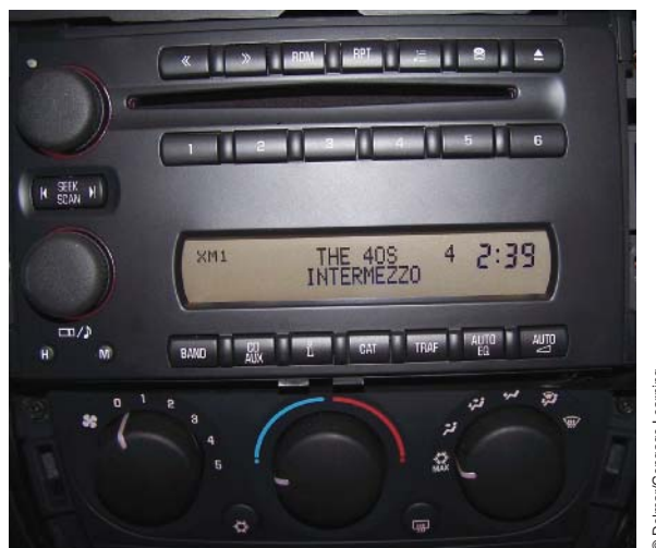
FIGURE 14-101 Satellite radio system.
