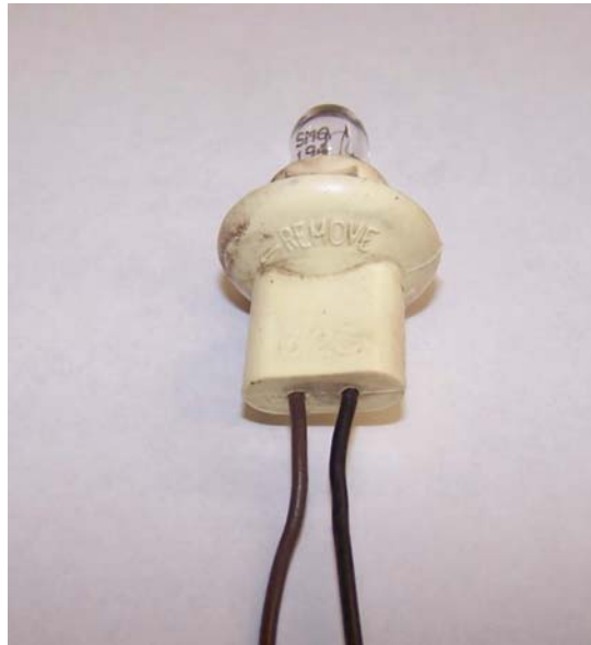
FIGURE 4-13 Molded connector halves are a one piece design that cannot be disassembled for repairs.
