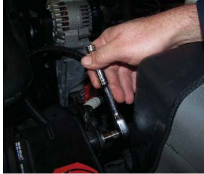
P24-2 Disconnect the battery negative cable.
