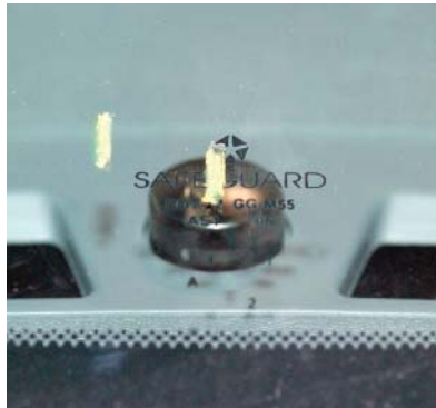
P22-5 Divide the lower measurement in half and mark that dimension near the upper edge of the blackout area using a grease pencil.
