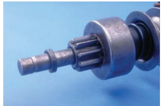
FIGURE 6-23 The pinion gear teeth are tapered to allow for smooth engagement.
