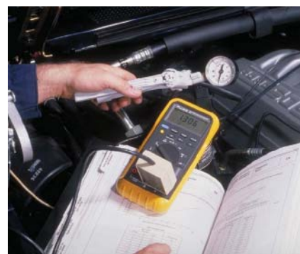
P19-6 Connect a hand vacuum pump to the MAP sensor and supply 5 in. Hg. Observe the MAP sensor reading and compare to specifications.
