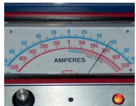
P12-9 The highest reading indicates maximum current output.
