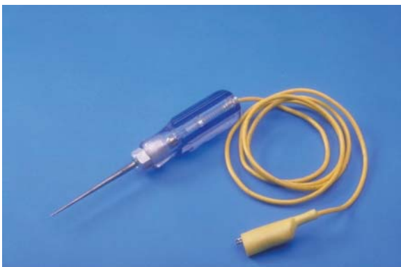
FIGURE 2-4 A typical test light used to probe for voltage in a circuit.
