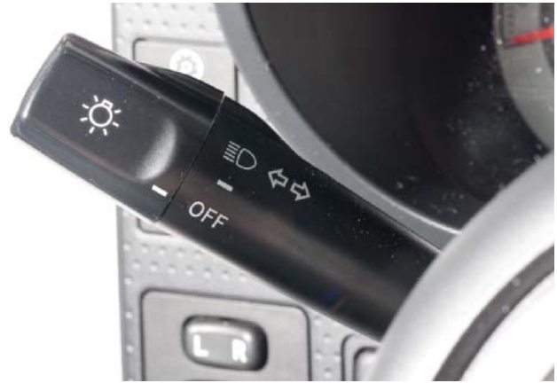
FIGURE 8-14 (A) Instrument panel-mounted headlight switch. (B) Steering column-mounted headlight switch.
