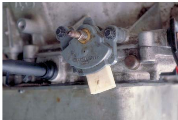
FIGURE 1-3 The neutral safety switch is usually attached to the transmission.
