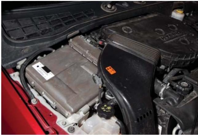
FIGURE 6-51 The inverter module controls the speed and direction of the AC motor.
