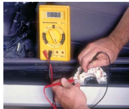
P16-15 With the switch in the high-beam position, continuity should be between terminals 15 and 12. Circuits 15 to 13, 196 to 13, and 196 to 12 should be open.
