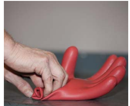
P2-3 Test the integrity of the insulating grooves prior to use. Wear the gloves until the high-voltage isolation procedure is complete.
