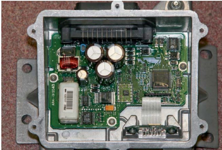
FIGURE 1-11 A control module is used to process data and operate different automotive systems.
