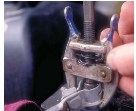
P16-3 Loosen the negative battery clamp bolt and remove the clamp using terminal pullers. Place the battery cable where it cannot contact the battery.
