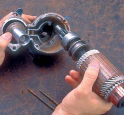
P10-10 Remove the armature from the drive housing. Note: On some units it may be necessary to remove the shift Clever from the drive housing before removing the armature.
