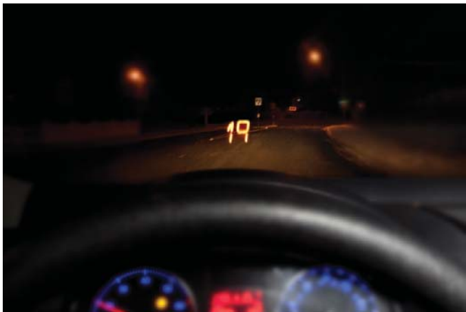
FIGURE 13-28 The HUD displays various information inside the windshield.
