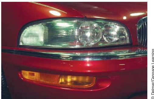
FIGURE 8-43 Wrap-around headlights serve as side marker lights.
