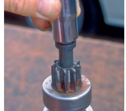
P10-12 Tap end of socket with a plastic hammer to drive the retainer toward the armature. Move it only far enough to access to the snap ring.
