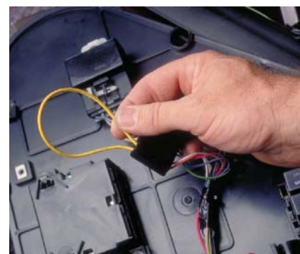
P27-3 Connect the jumper wire between terminals A and B. The horns should sound.
