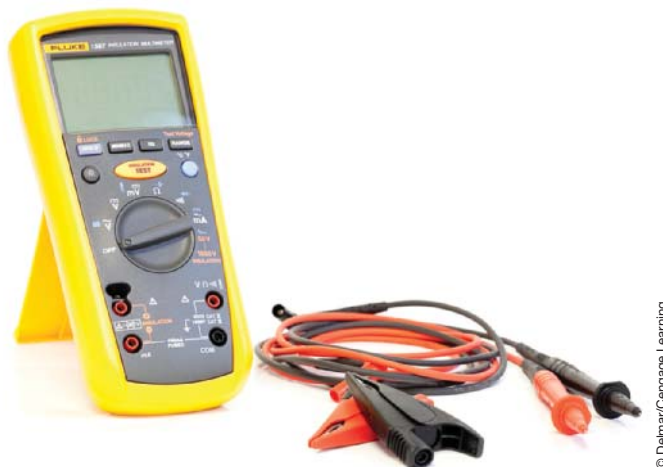
FIGURE 2-23 An insulation meter is used on many HEVs to determine insulation leaks in the high-voltage system.
