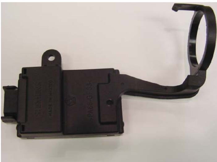
FIGURE 14-72 The immobilizer module with halo antenna.
