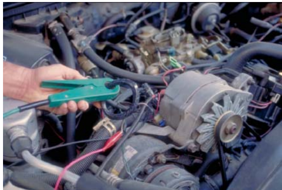
FIGURE 7-7 Connecting the multiplying coil and amp pickup to a generator.
