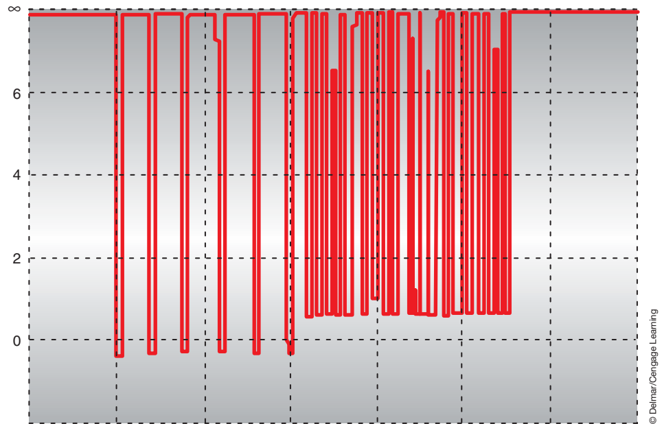
FIGURE 11-3 ISO K data bus transmission voltages.
