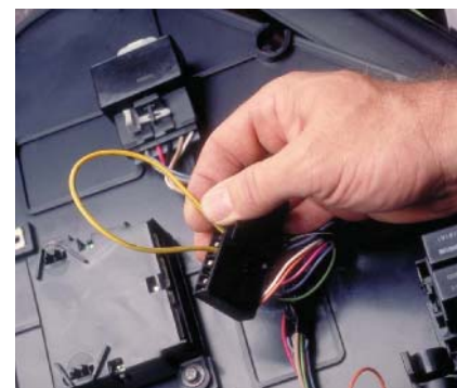
P27-6 Connect the jumper wire between terminals D and E.
