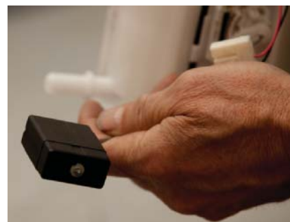
P23-9 Check the float that it is not filled with fuel, distorted, or loose.
