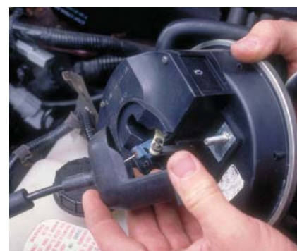
P28-9 Remove the two cable cover to servo assembly retaining bolt and pull off the cover.
