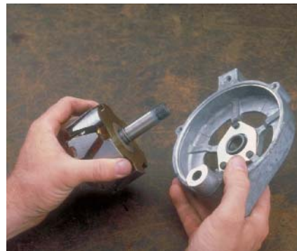
P14-15 Separate the front housing from the rotor. If the stop ring is damaged remove it from the rotor, if not leave it on the rotor shaft.
