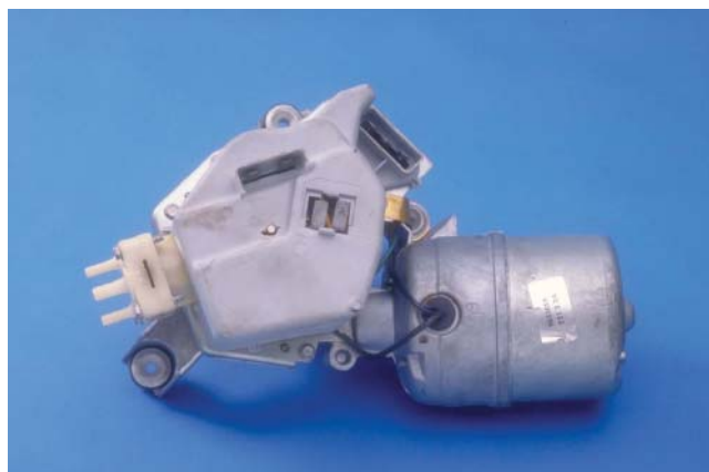
FIGURE 14-29 General Motors' pulse-type washer system incorporates the washer motor into the wiper motor.
