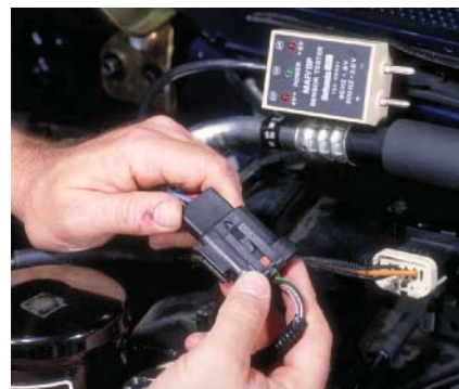
P19-3 Connect the MAP sensor connector to the harness connector.
