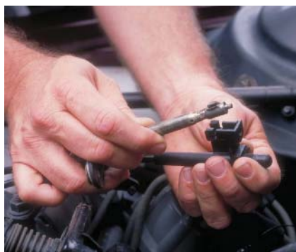
P28-4 Disconnect the speed control cable from the accelerator cable.
