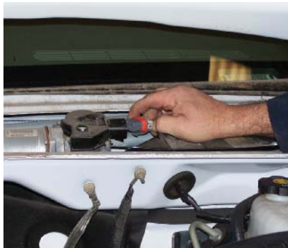
P24-5 Disconnect the wire connector at the motor.
