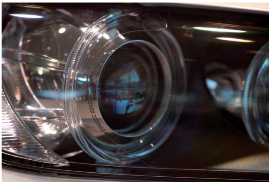
FIGURE 12-16 The adaptive headlight assembly use motors to rotate the beam.
