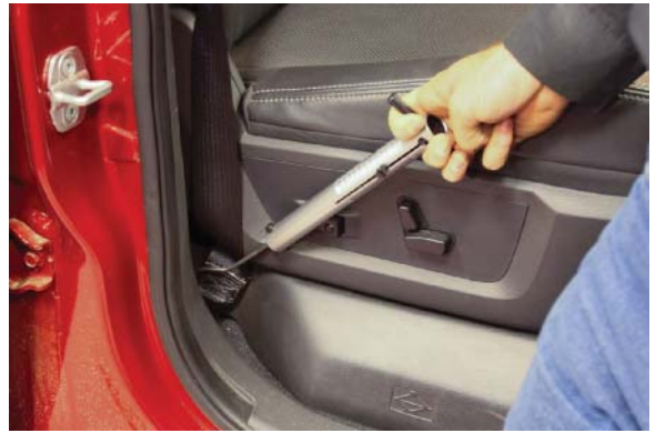
FIGURE 15-12 Using the pull scale to obtain pressure against the BTS.
