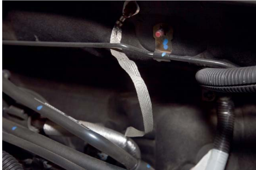
FIGURE 4-4 Ground straps are used to provide a return path for components that are insulated from the chassis.
