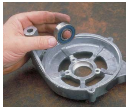
P14-18 Remove the front bearing from the housing. NOTE: It may be necessary to use an arbor press to remove the bearing if it does not slide out.
