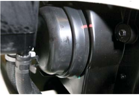
FIGURE 8-4 The HID element is protected by a rubber boot on the back of the headlight assembly.
