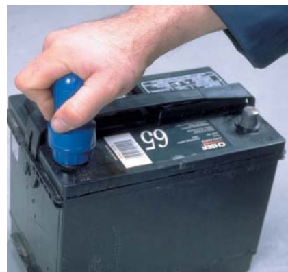
FIGURE 5-9 A terminal cleaning tool is used to clean the battery's terminals and the cable's clamps
