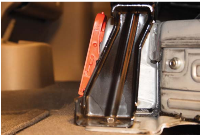
FIGURE 1-31 The high-voltage service plug is usually located near the HV battery.
