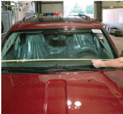
P22-4 Measure across the upper edge of the blackout area at the bottom of the windshield using the inside corner of the intersection between the side blackout area and the lower blackout area as the reference points.
