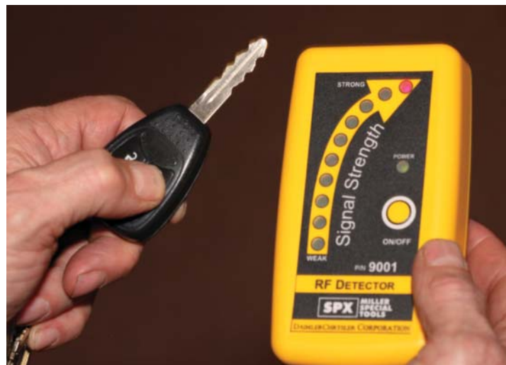
FIGURE 14-29 RF signal meter indicates the strength of the signal.
