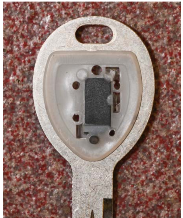
FIGURE 14-73 The immobilizer key has an internal transponder chip. The key cover was cut off for this illustration.
