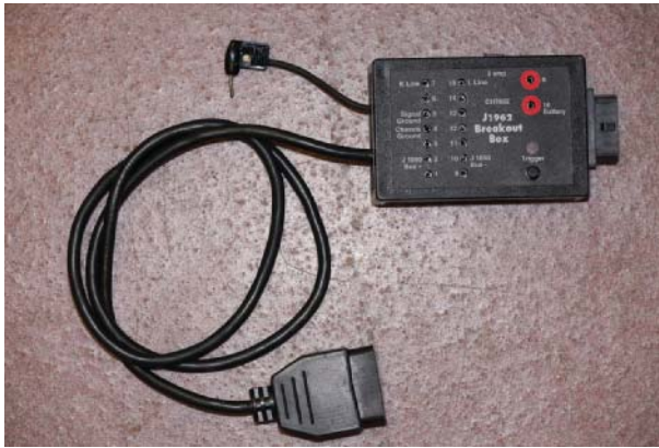
FIGURE 11-1 The J1962 BOB makes pin out testing of the DLC easier.
