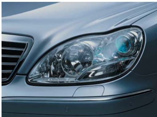
FIGURE 8-9 HID headlamps; note the reduced size of the headlamp assemblies.
