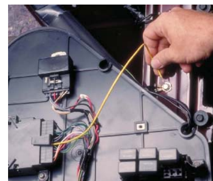
P27-9 Connect the jumper wire from terminal F to a good ground.
