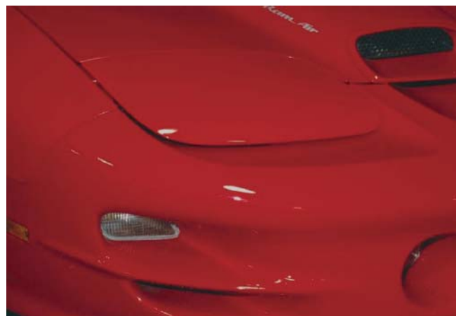
FIGURE 8-20 Concealed headlights enhance the vehicle's styling and aerodynamics.
