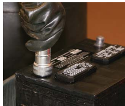
P9-15 Use the cleaning tool to clean the battery posts.
