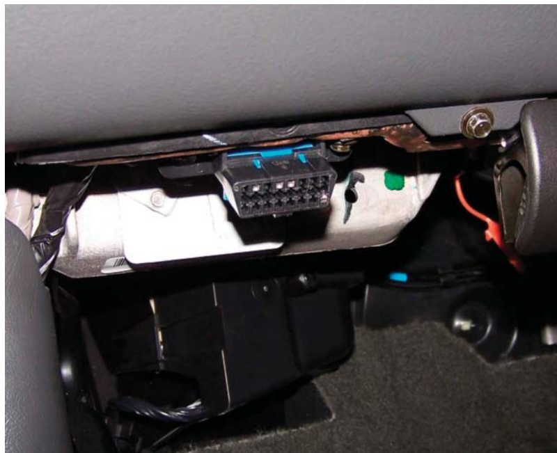
FIGURE 2-36 The scan tester connects to the diagnostic link connector (DLC).
