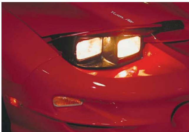
FIGURE 8-20 Concealed headlights enhance the vehicle's styling and aerodynamics.
