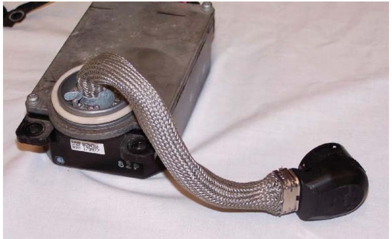
FIGURE 8-5 The ignitor is connected to the ballast by a cable.
