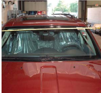
P22-2 Using the “ASI” marks on both sides of the windshield, measure across using the shaft of the tint band arrow as the reference points.
