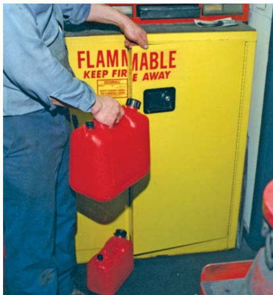
FIGURE 1-20 Store any type of combustible materials in an approved safety cabinet.
