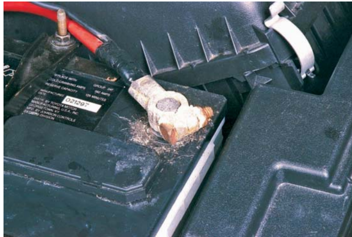
FIGURE 5-4 Inspect the condition of the battery cables and terminals.
