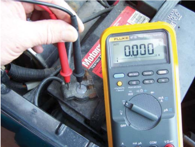
FIGURE 5-7 Voltmeter connections for the battery terminal test.
