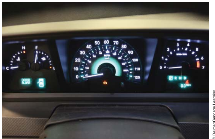
FIGURE 13-10 Electronically controlled swing needle instrumentation.
