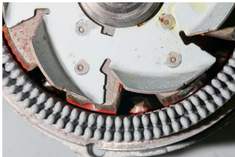
FIGURE 7-13 A small air gap between the rotor and the stator maximizes the magnetic force.
