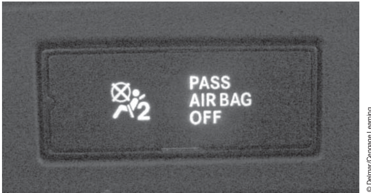
FIGURE 15-37 The PADL illuminates if the air bag is suppressed.
