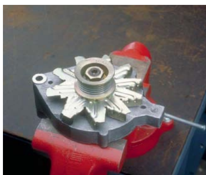
P14-13 Clamp the rotor in a soft jaw vise.
