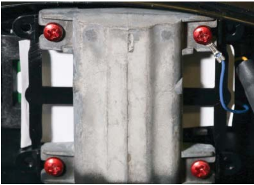
FIGURE 12-8 An adjustment shim is used to align the camera.
