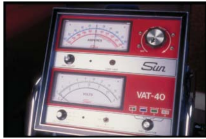
FIGURE 5-1 A Sun VAT-40 battery, starting, and charging system tester.
