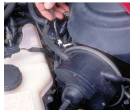
P28-6 Remove the two retaining bolts that attach the servo assembly bracket to the shock tower.
