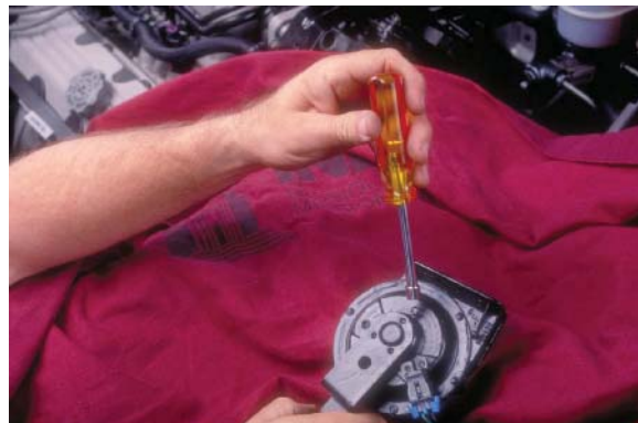
FIGURE 14-3 Horn pitch adjustment screw.
