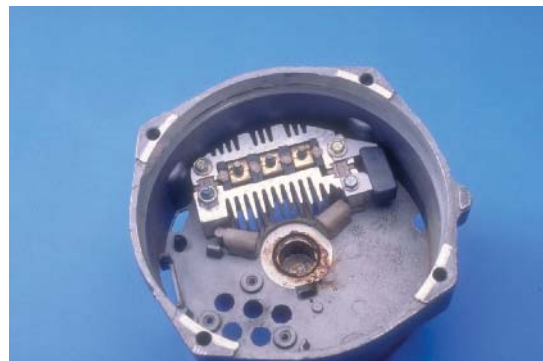
FIGURE 7-17 General Motors' rectifier bridge.
