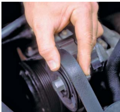
P13-2 The belt must be replaced if it is glazed.
