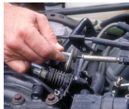
P28-3 Disconnect the cable from the brackets.
