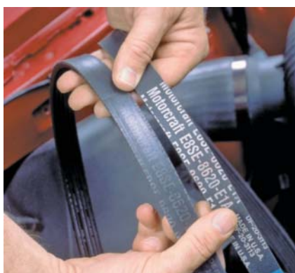
P13-7 Confirm that the new belt is the same size as the old one.
