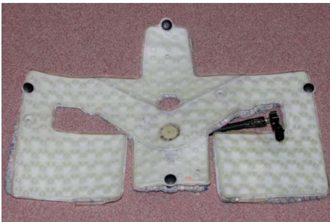
FIGURE 15-38 Bladder used to determine occupant classification.
