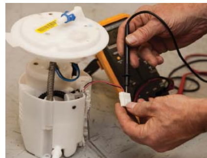
P23-3 Connect the negative test lead DMM to the ground terminal of the sender unit.
