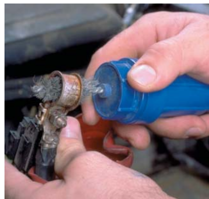
FIGURE 5-9 A terminal cleaning tool is used to clean the battery's terminals and the cable's clamps
