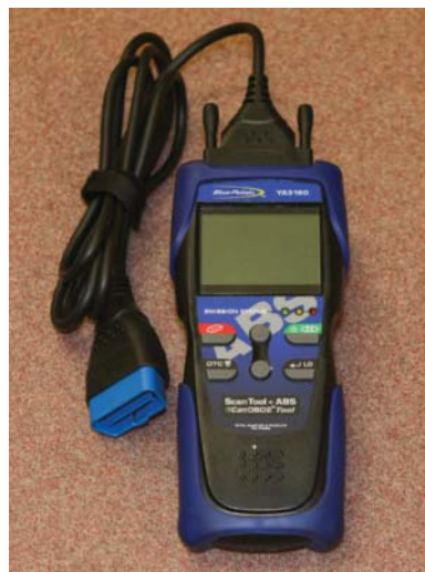
FIGURE 9-9 A scan tester is used to enter the computer's diagnostic capabilities.
