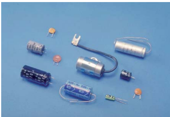
FIGURE 2-36 Capacitors that can be used in automotive electrical circuits.
