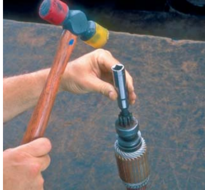
P10-11 Place a 5/8" deep socket over the armature shaft until it contacts the retaining ring of the starter drive.
