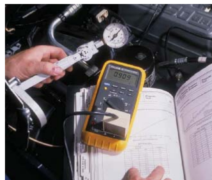
P19-9 Increase the vacuum 20 in. Hg to the MAP sensor and compare the reading to specifications. If any of the MAP sensor readings do not meet specifications, replace the MAP sensor.
