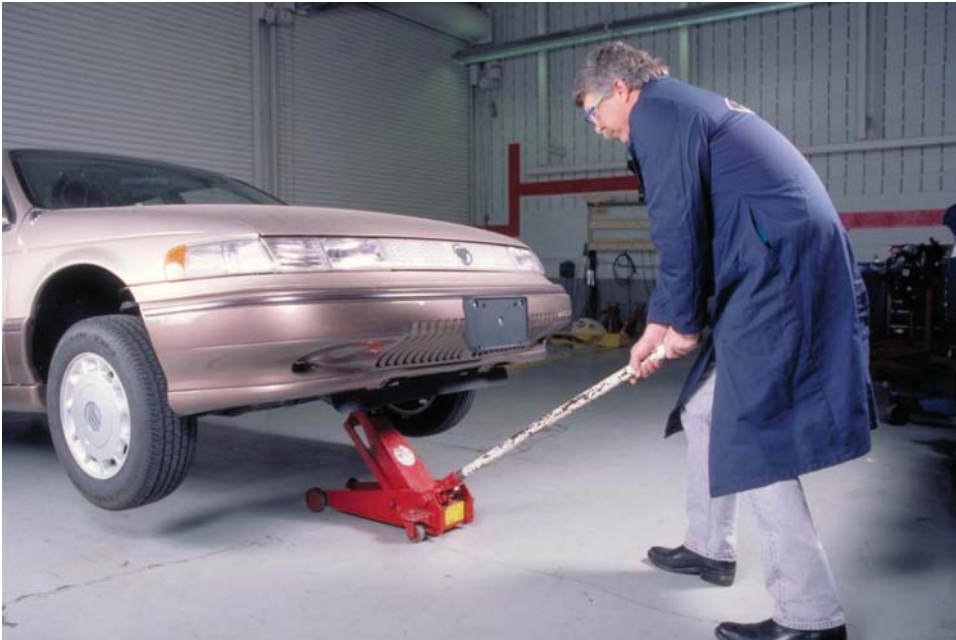
FIGURE 1-6 Floor jacks are used to raise the vehicle a short distance off the floor.
