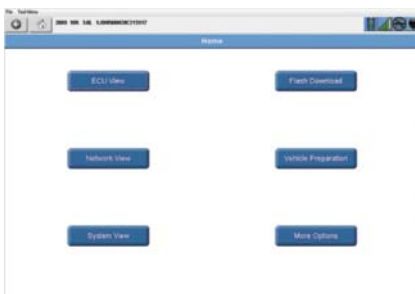
P20-1 The “Home” screen of the scan tool. Select “Network View.”
