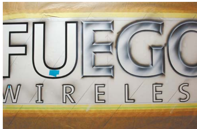
Left: Here is why you had the sign shop cut two stencils. Place the inside pieces of the letters over what has been airbrushed so far. If you are using a hand-cut stencil, use the pieces you saved from the earlier step. Place the pieces over the letters covering what was airbrushed. Right: This photo shows the result of the step I'm about to do next. The uncovered area around the letters will become the beveled edge. The letters on the right have had the bevels airbrushed. The next photos show how to airbrush that edge.
