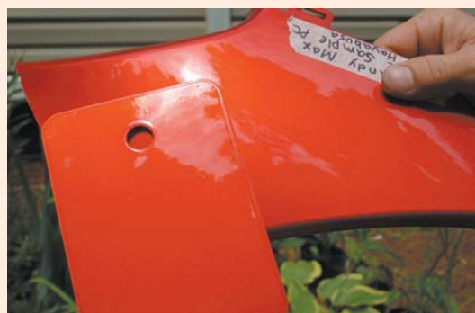
Looking at a color from a straight on angle in direct sunlight, the color looks nice and bright. The color sample appears to be a perfect match to the original color.
