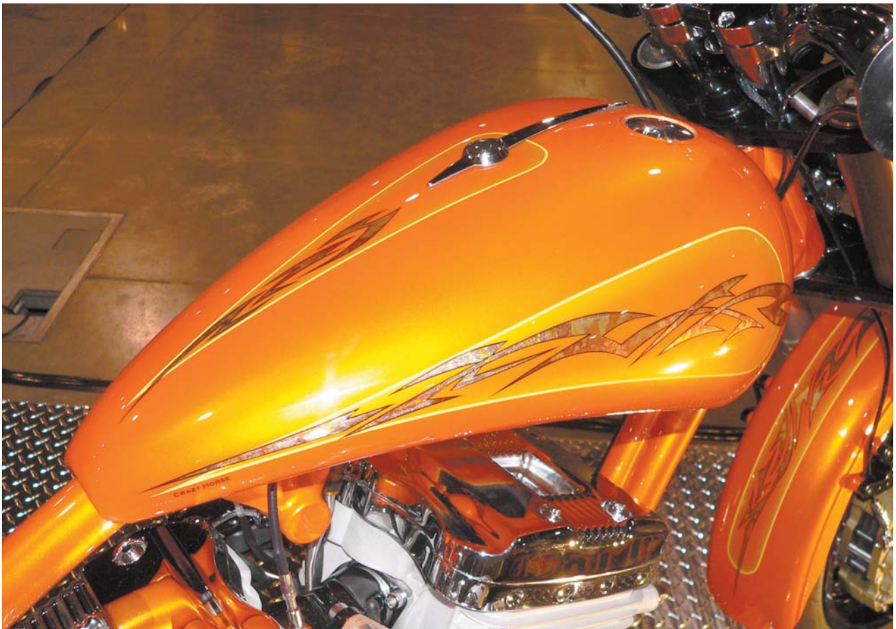
A number of elements combine to create this eye-catching paint job: properly done bodywork, color testing to create the basecoat color, pre-paint drawings to find the most effective design, and a thorough knowledge of the materials and tools used.
