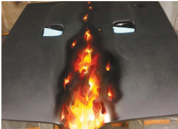
The real fire flame artwork has been completed on the Firebird. Now it must be clearcoated to protect and level out the layers of the artwork.
