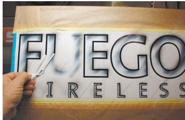
Left: I airbrushed the white edges very lightly with white once more. Don't overdo this step. Right: Next, I peeled off the outer border of the stencil lettering.
