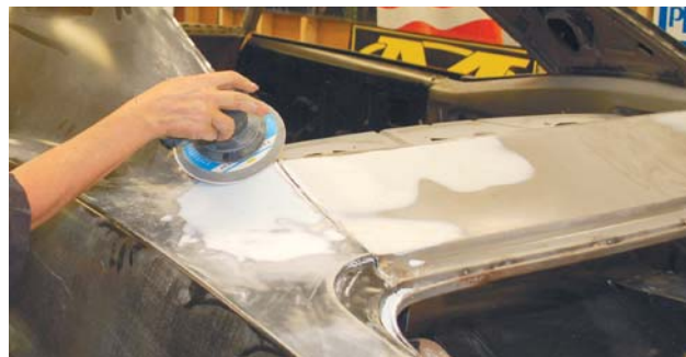
I used a DA and 80 grit to rough out the filler.
