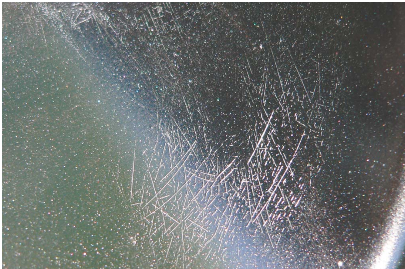
Notice the slight lines running across this surface? They are actual cracks in the paint.
