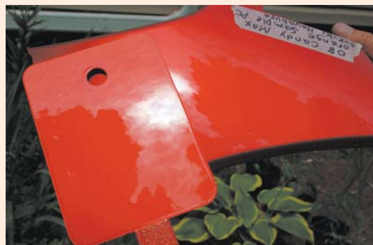
But when viewed in the shade from a slight angle, the sample flops dark—darker than the color. It's not a big difference, but it's enough of a difference to be noticed as not matching.
