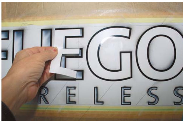
Left: Here is why you had the sign shop cut two stencils. Place the inside pieces of the letters over what has been airbrushed so far. If you are using a hand-cut stencil, use the pieces you saved from the earlier step. Place the pieces over the letters covering what was airbrushed. Right: This photo shows the result of the step I'm about to do next. The uncovered area around the letters will become the beveled edge. The letters on the right have had the bevels airbrushed. The next photos show how to airbrush that edge.
