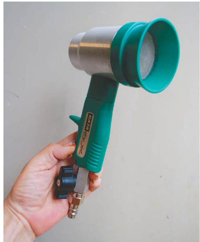
The SATA dry jet is perfect for helping dry the water out of the paint. It's more of an air diffuser than an air gun.
