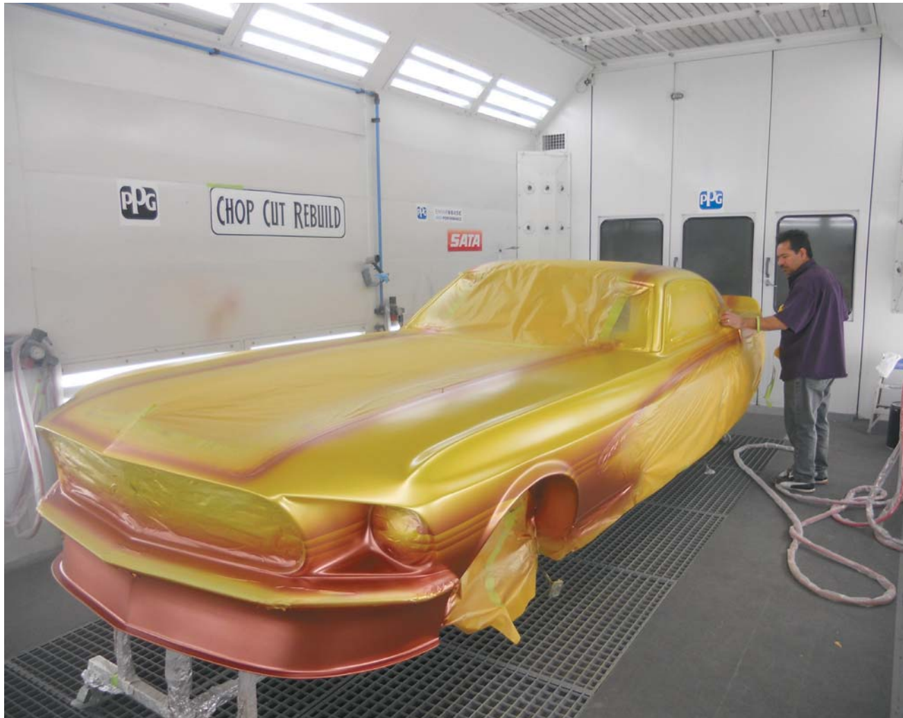
Paint booths now feature fans or blowers to move air in a way that helps dry the water out of waterborne paint. This booth has been retrofit with a drying blower and turbulent air system tower in each corner of the booth. These provide clean, filtered air, which helps promote a controlled flash off of waterborne basecoats and rapid curing of low-VOC topcoats.
