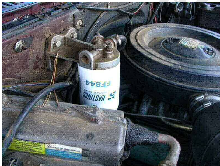
A fuel filter (white) next to the air filter compartment (circular black part)
