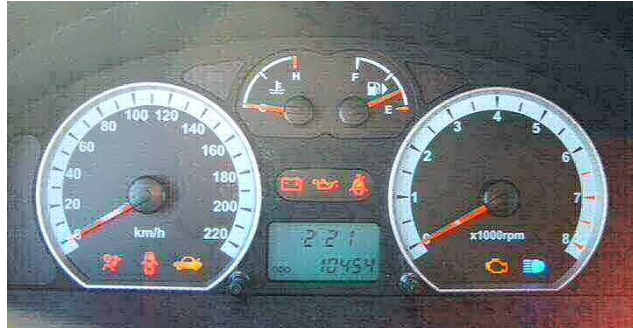
Dashboard showing gauges and warning indicator lights Image credit: CC-BY-SA-Tagaz Vega
