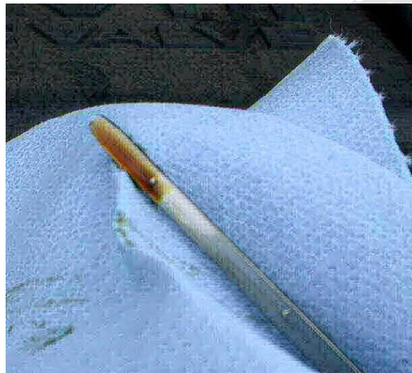
Oil dipstick (above) and oil level on a dipstick (below) Image credits: both CC-BY-SA-Dvortygirl on Wikipedia
