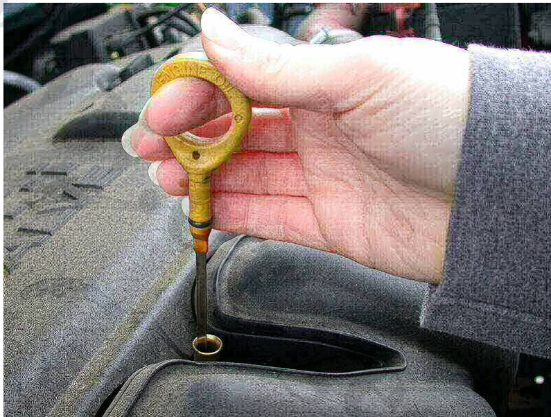
Oil dipstick (above) and oil level on a dipstick (below) Image credits: both CC-BY-SA-Dvortygirl on Wikipedia
