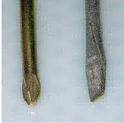
Screwdriver tips showing Philips (left) and flat or slotted (right)
