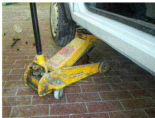
Hydraulic jack with hand-pump mechanism
