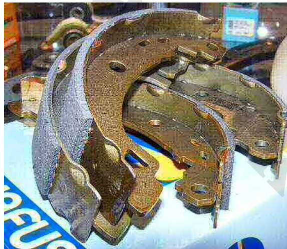
Drum brake shoes (violet color) and linings.
