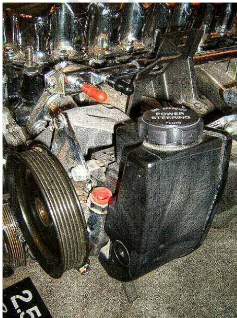
Power steering reservoir (black tank). Notice how the cap is labeled.
