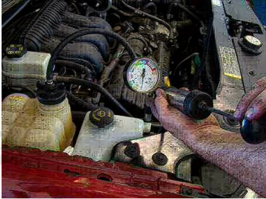
Pressure testing the cooling system
