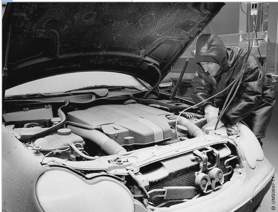
4 Recording cold-starting response in the cold room
