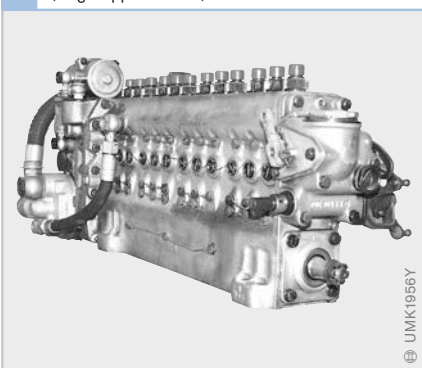
13 12-cylinder in-line fuel-injection pump (length approx. 70 cm)
