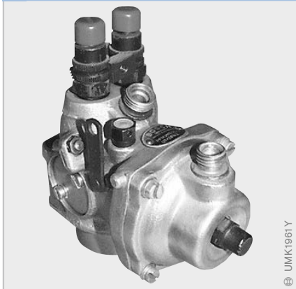
18 Two-cylinder fuel-injection pump (length approx. 15 cm)
