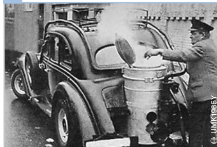
22 Wood-gas generator system on a 1936 Adler Diplomat
