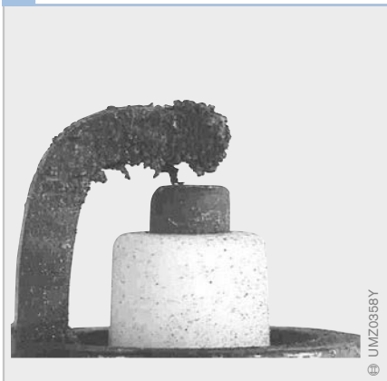
2 Ground electrode damaged from excessive knock
