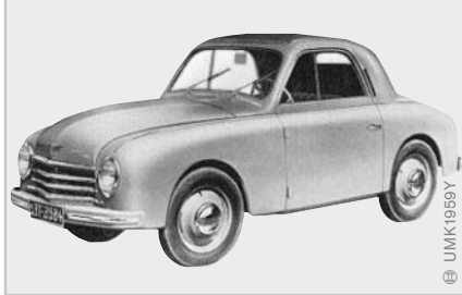
17 Goliath GP700E (1951–1957; after 1954 with direct injection)
