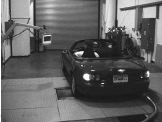
FIGURE 12.3 Test vehicle inside an EPA test facility. (Reproduced from Environmental Protection Agency. Available at www.fueleconomy.gov/feg/fe_test_schedules.shtml .)
