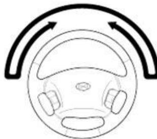
Checking steering wheel return
