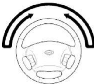
Checking steering wheel return
