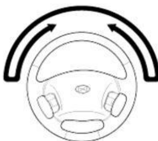
Checking steering wheel return
