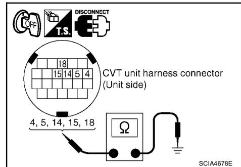
2. If NG, check continuity with control cable disconnected. (Refer to step 1 above.)
