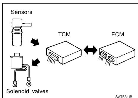
It is much more difficult to diagnose an error that occurs intermittently rather than continuously. Most intermittent errors are caused by poor electric connections or improper wiring. In this case, careful checking of suspected circuits may help prevent the replacement of good parts.
