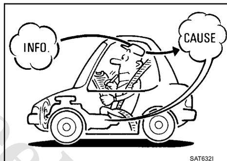
Before undertaking actual checks, take a few minutes to talk with a customer who approaches with a driveability complaint. The customer can supply good information about such errors, especially intermittent ones. Find out what symptoms are present and under what conditions they occur. A "DIAGNOSTIC WORKSHEET" as shown on the example (Refer to [CVT-27](#)) should be used.
