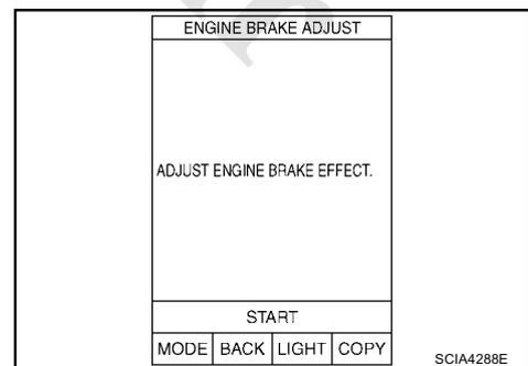
4. Set "ENGINE BRAKE LEVEL" by touching "UP" or "DOWN".
