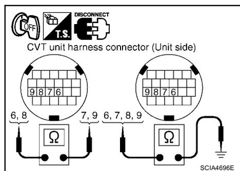
4. If NG, replace the transaxle assembly. Refer to [CVT-153, "Removal and Installation"](#).
