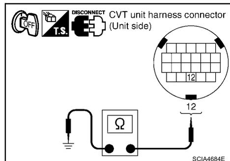
**DTC P0744 A/T TCC S/V FUNCTION (LOCK-UP)**
