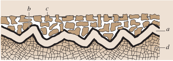
Fig. 5.16 Solid lubrication made of lubricating varnish: a: phosphate layer (3 \mu\text{m} ); b: binder; c: solid lubricant; d: base metal (after [5.16])
