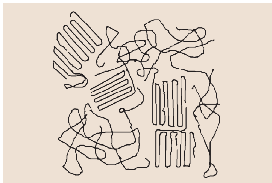
Fig. 3.161 Amorphous and crystalline regions in the morphology of a semicrystalline polymer
