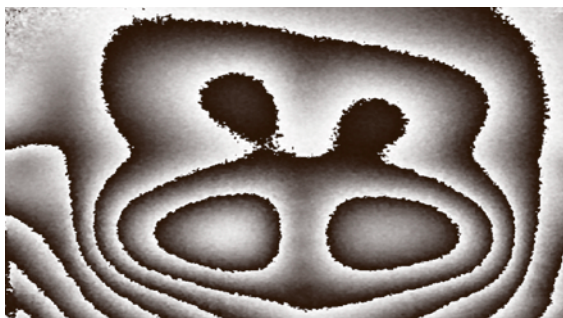
Fig. 3.99 Speckle fringes caused by discontinuities of off-plane surface displacements
