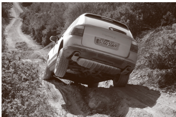
Fig. 13.84 Test with sports utility vehicle to verify performance under extreme road conditions (courtesy of Dr. Ing. h.c. F. Porsche AG)
