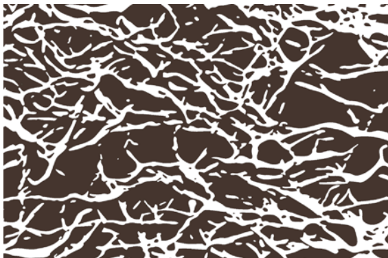
Fig. 5.17 Fiber structure of a grease with soap thickener [5.19]
