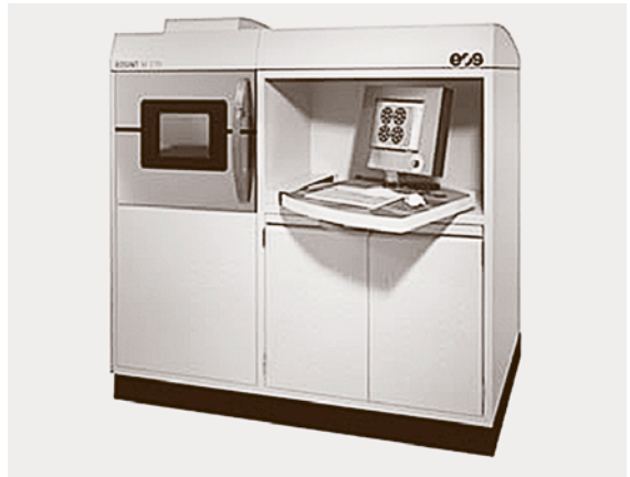
Fig. 7.334 EOSINT M270 – EOS device. Technical characteristics: materials: tool steel H20, steel DS20, Ti6AL4V, stainless steel EOS 17-4 PH, bronze DM20; full melting; layer thickness 20–100 \mu\text{m} ; accuracy 0.05–0.1 mm; build volume 250 \times 250 \times 215\text{ mm} ; speed 5–70 \text{cm}^3/\text{h}
