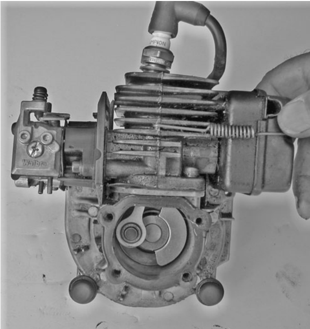
FIG. 1-6. Carburetors for third-port engines attach to the cylinder. Some of these engines incorporate a reed valve in the third port. Robert Shelby
