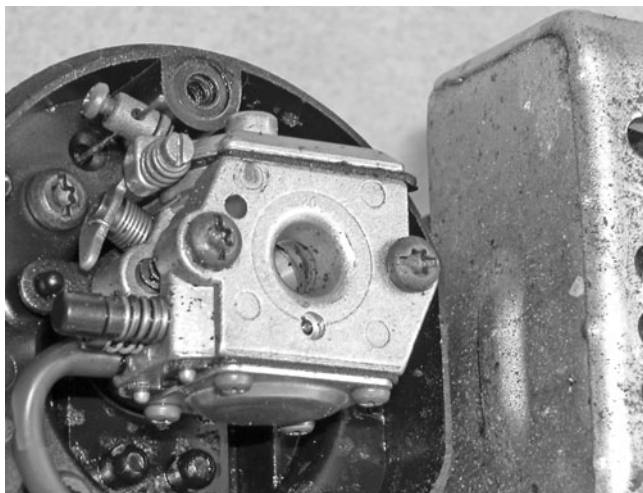
FIG. 2-9. Carburetors often vibrate loose from their mounts and leak air. Robert Shelby
