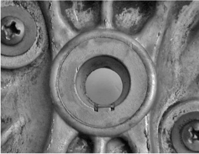
FIG. 3-6. Flywheels with stripped cast-in keys can be salvaged with a suitable file and patience. Robert Shelby
