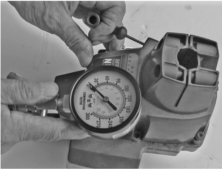
FIG. 2-11. Cylinder compression is a basic indication of engine health. Robert Shelby
