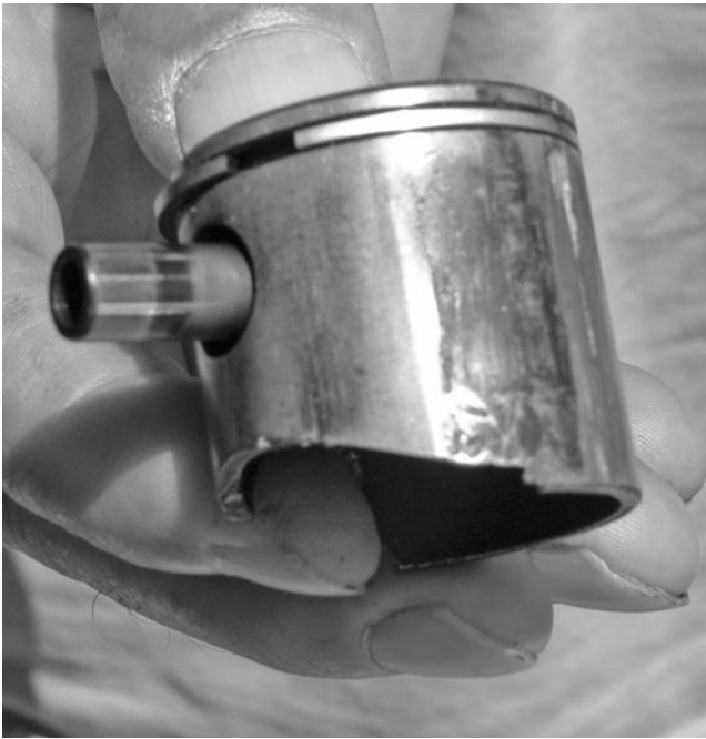
FIG. 2-8. High combustion temperatures are death on pistons. This example exhibits pock marks left by metal fragments, deep scores, and, near the crown on the right of the photo, weld splatches. Robert Shelby
