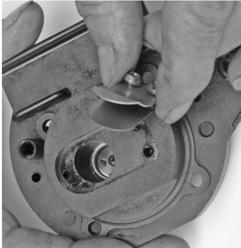
FIG. 1-3. Reed valves for handbeld engines generally have a single pedal backed by a guard plate to limit deflection. Robert Shelby
