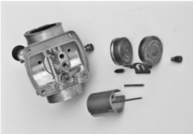
FIG. 4-34. The throttle consists of a tubular slide with a cutaway on the leading edge. The needle moves with the slide to vary fuel delivery in concert with air flow. A “pontoon” float is pretty well standard, in the tradition of early Amal units. Robert Shelby
