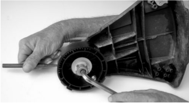
FIG. 7-12. Most trimmer heads can be locked with a small punch. Robert Shelby
